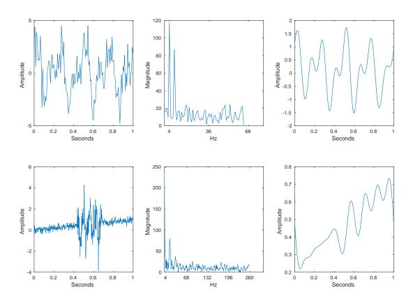
The figure above shows two different 1-D signals (left column) with their corresponding spectrum obtained using the FFT (middle column). In the right column, we show a signal obtained by discarding part of the frequencies in the spectrum.
